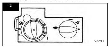
• Ensure that the left-hand control knob is pointing to off (  ${\ensuremath{\bullet}}).$
